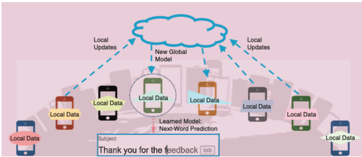
Figure 9: Demonstration of federated learning with mobile phones held by individual users as devices. Adapted from [Li+20].
